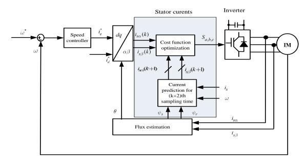
Figure 2. Block structure of the stator current controllers with predictive current controller
