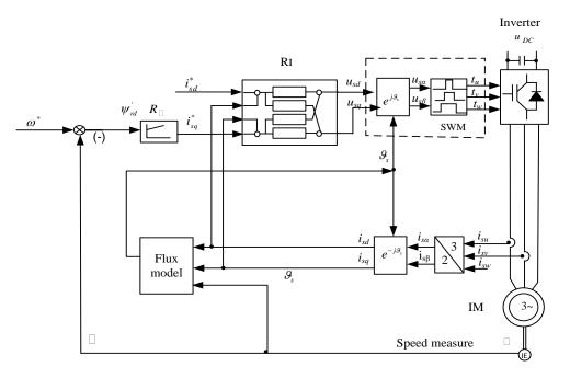
Figure 1. Block structure of the PI stator current controllers
