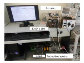
Figure 3. Photo of experimental setup
