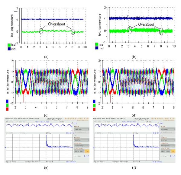
Figure 4. Stator current responses, (a) Stator current response using PCC-FOC, (b) Stator current response using PI-FOC, (c) 3 phase stator current response PCC-FOC, (d) 3 phase stator current response PI-FOC, (e) Total harmonic distortion (THD%) PCC-FOC, (f) Total harmonic distortion (THD%) PI-FOC
